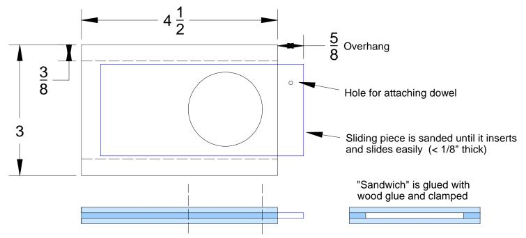
Use glue sparingly so no glue oozes out of the sandwich into the interior of the slide case.
